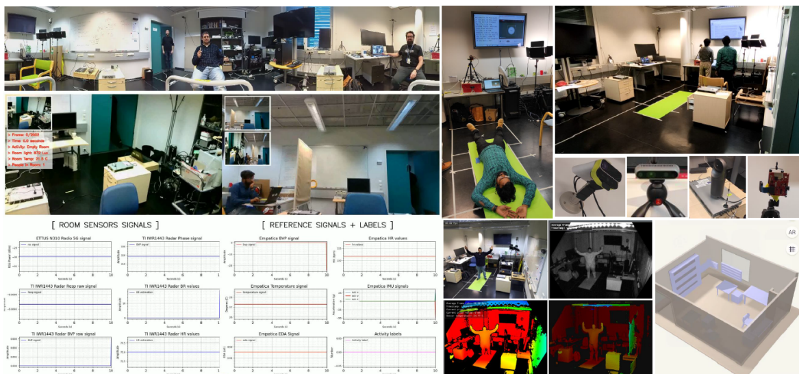
Figure 6 - Sensorized indoor room with multiple cameras (visual) and communication devices (radios) which form the input data for the environment modeller.
