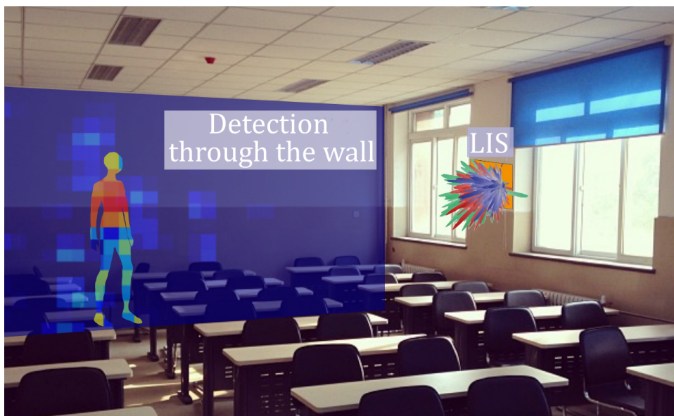
Figure 12 - UC1.3: An example scenario using a LIS-assisted radar for RF mapping of targets hidden behind a wall.
